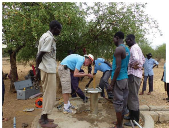
W4EE team member Mike Wood provides hand-pump management training in Napotpot, Kapoeta East County, Kapoeta State, to measure static water level in boreholes as part of groundwater monitoring.
